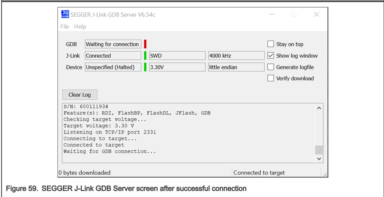
Figure 59. SEGGER J-Link GDB Server screen after successful connection
