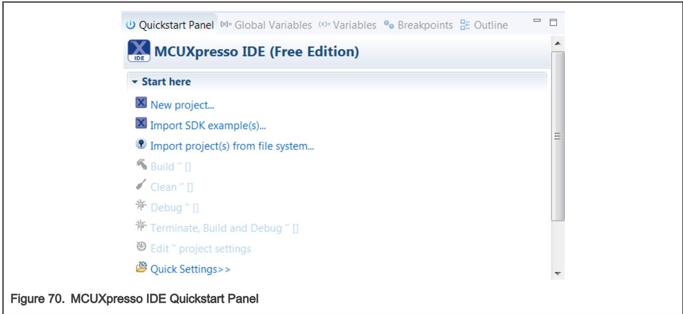
Figure 70. MCUXpresso IDE Quickstart Panel
